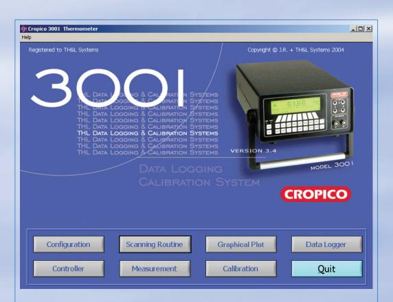
The purpose of the Model 3001 software is to provide easy to use and accurate temperature measurement, Data Logging and automated temperature calibration.
